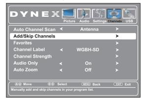
3 Press ▲ or ▼ to highlight Add/Skip Channels, then press ENTER. The channel list opens.
